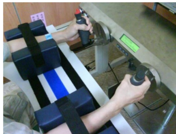
Figure 3 Bilateral robot-assisted training is shown with the Bi-Manu-Track.
