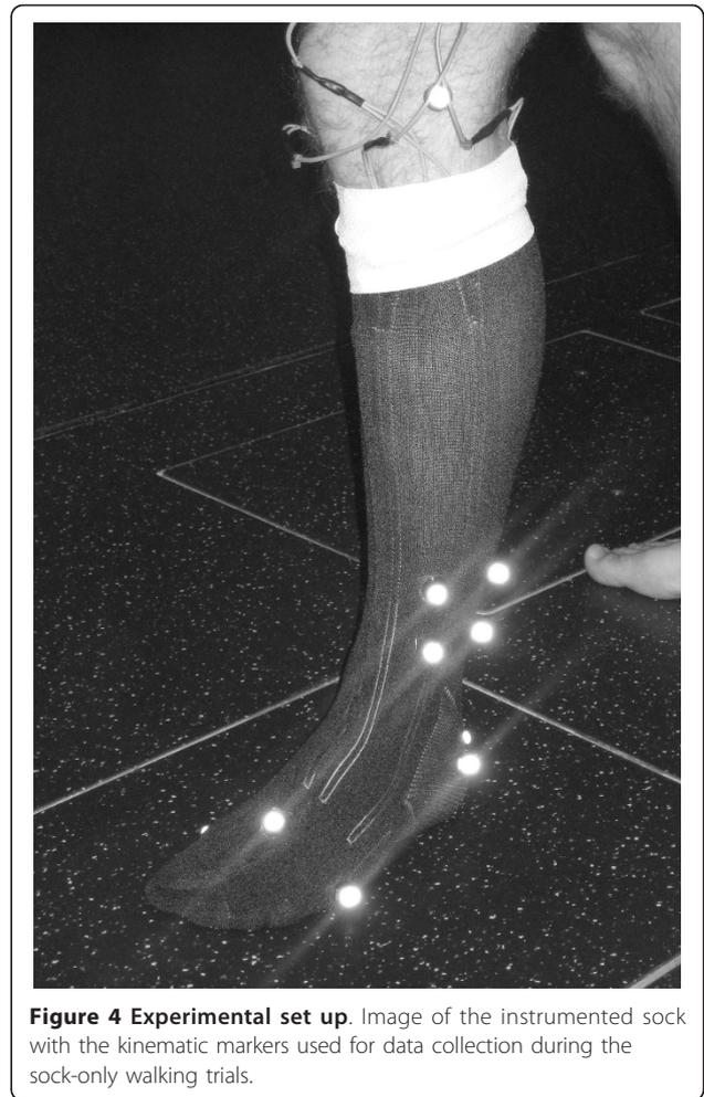
**Figure 4 Experimental set up.** Image of the instrumented sock with the kinematic markers used for data collection during the sock-only walking trials.
